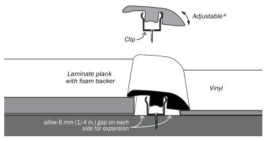
$<sup>^{\</sup>star}$  Adjust the position of the moulding in the clip based on the height of the lower surface flooring
